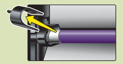
2.Turn old UV lamp until pins line up with housing slot.
